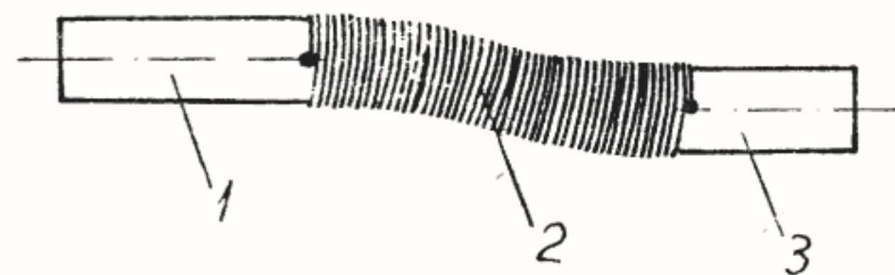
Fig. 55 — Cuplaj elastic: 1. ax motor; 2. resort; 3. ax port elice.
